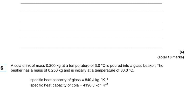
(i) Show that the final temperature,  $T_f$ , of the cola drink is about 8 °C when it reaches thermal equilibrium with the beaker. Assume no heat is gained from or lost to the surroundings.
